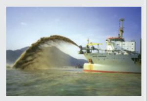
Fig. TB2.10.4. A trailing suction hopper dredger from the Netherlands similar to the type used for the reclamation of the new Hong Kong International Airport in action in Hong Kong. Sand is placed hydraulically using a technique known as rainbowing (© W.W.-S. Yim)
